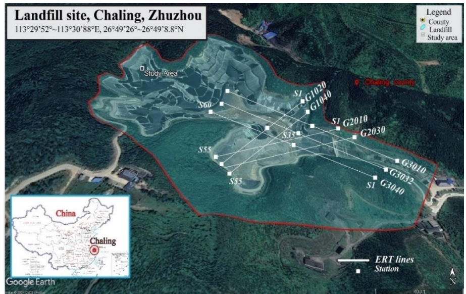
Figure 14: Overview of the Chaling Landfill Site and Study Area. The main map highlights the study area boundary (red outline), showing the distribution of Electrical Resistivity Tomography (ERT) lines (G1020, G1040, G2010, G2030, G3010, G3032, G3040) and stations (S1, S55, S60, S35) used in the study.
