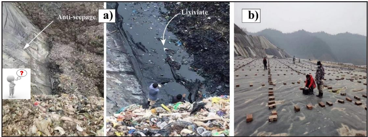
Figure 15: Field Operations at Chaling County Landfill. This series of images showcases various stages of landfill management and ERT exploration at Chaling County. From left to right: the accumulation of waste materials at the landfill site, a worker conducting ERT data collection amidst the debris, and the setup of an extensive ERT exploration grid over a covered section of the landfill. These scenes depict the practical challenges and efforts involved in environmental monitoring and management.
