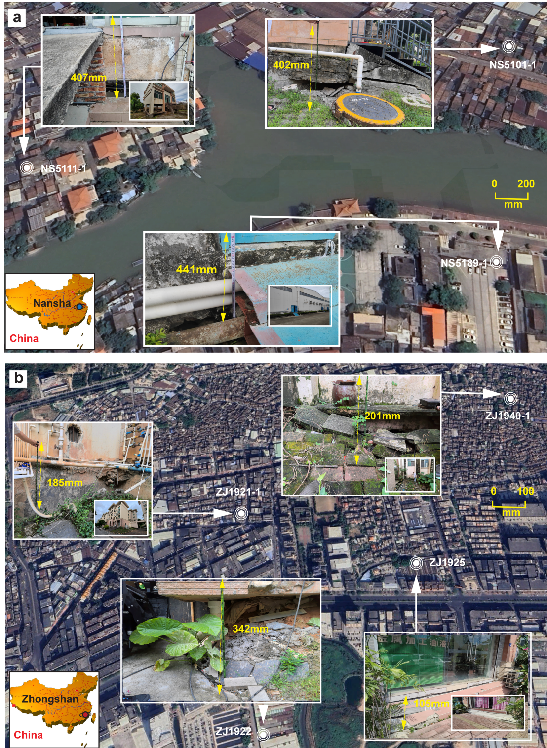
图 3-1 Field evidence of differential settlement in Nansha and Zhongshan. a , Nansha: oblique satellite view with locations of selected InSAR pixels (NS5111-1, NS5101-1, NS5189-1) and photographs of nearby buildings. Yellow arrows indicate vertical offsets between building plinths and the surrounding ground, with measured gaps of approximately 402–441 mm at several riverfront structures. b , Zhongshan: similar layout for pixels ZJ1921-1, ZJ1922, ZJ1925 and ZJ1940-1, illustrating tilted walls, uplifted steps, and exposed foundations with offsets of roughly 105–342 mm. Insets show the wider building context. These field observations corroborate the persistent subsidence hotspots identified by the InSAR time series in both cities.
